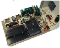
The HEMOX Analyzer consists of the main console which is a sheet metal housing, upon the base of which the optical and electronic components are mounted. Also contained in the housing is the gas selection valve system and the pumping system for sample intake and removal.
