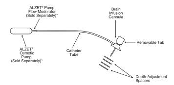
\* The ALZET Brain Infusion Kit has been designed specifically to work with ALZET osmotic pumps. For further information on ALZET pumps, please contact ALZET Technical Support at (800) 692-2990 or (408) 367-4036.
